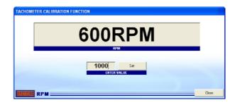
Enter an RPM value in the box marked ENTER VALUE, the press the SET button. The tachometer LED will illuminate – point the optical tachometer at the LED.
