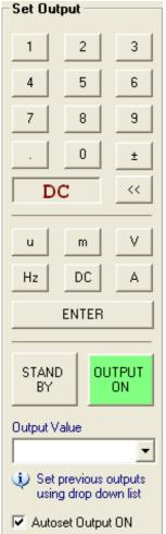
The Set Output panel, shown left, allows the user to select a value to output and then automatically set the calibrator output and switch to the appropriate terminals on the workstation adapter.
